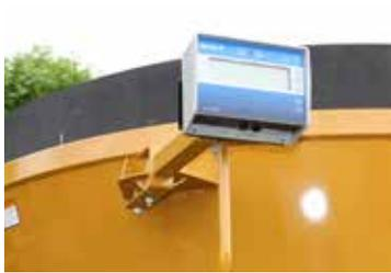
**Digi-star:** The CMF-590 is equipped with a Digi-Star 4 pt. scale and monitor. Various monitor options are available. The Digi-Star system is powered by a standard onboard 12-volt battery. Digi-Star feed rationing programs are also available.
