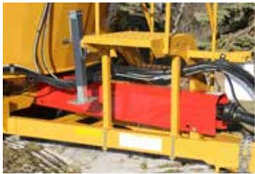
**CV PTO:** The CMF-590 comes equipped with a Heavy-Duty Constant Velocity 1000 rpm PTO. The 2-Speed Gear Box is used for loaded start-ups and heavy rations.
