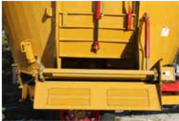
**Magnets:** Magnets on the discharge chutes remove metal, such as bale wire, from feed providing protection for your cows.
