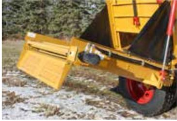
**Conveyor:** The unloading door is 42" wide and can be on the left or right side of the machine. Conveyor options are a 3' or 5' extension which gives a feeding height range of between 40" and 62".
