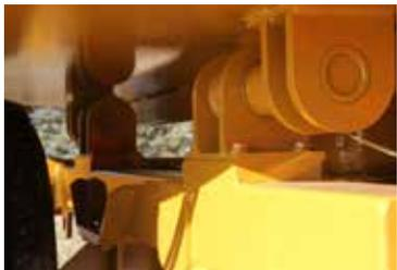
**4-Point Scale:** 4-point scale for accurate weighing, with reduced scale bounce during loading and feeding
