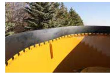
**Rubber extension:** The tapered boil ring is standard equipment on the CMF-590. It prevents product from boiling over the sides during the cutting and mixing processes.
