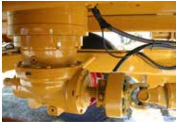
**Clutch:** Free motion clutches on the driveline protect the heavy-duty gear boxes. Gear boxes come with a 2-year warranty.
