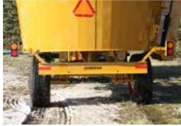
**Rigid Axles:** Rigid heavy-duty axles on 2 385/65R 22.5 tires.
