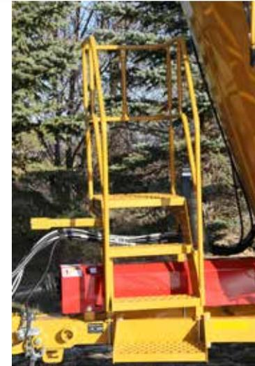
**Ladder:** Ladder mounted on front of machine allows for viewing of mixed ration. The ladder should only be used while the machine is stopped.
