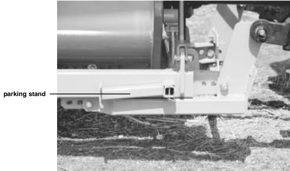
Figure 3.5 Location of parking stand, shown in transport/working position
