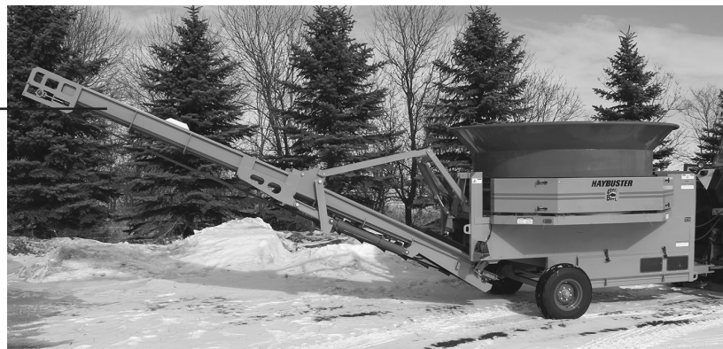
conveyor in working position
