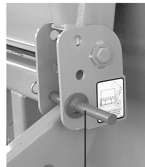
loader transport pin in storage position
