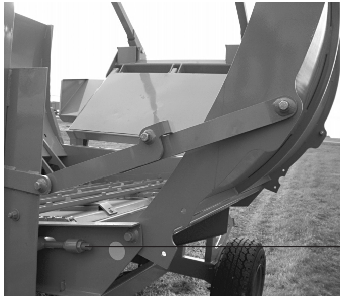
Bale conveyor chain tightener
