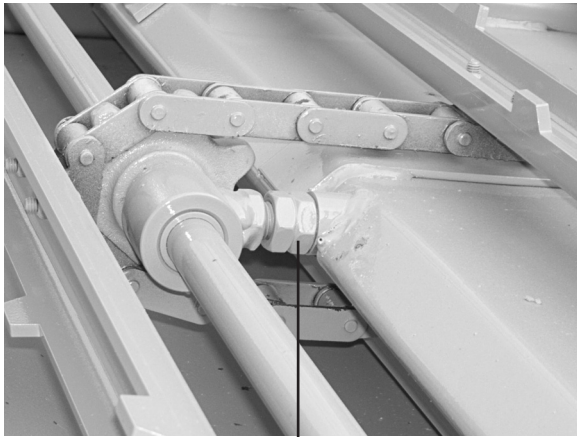
center conveyor chain adjustment bolt
