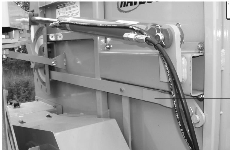
Rack tool in stored location
