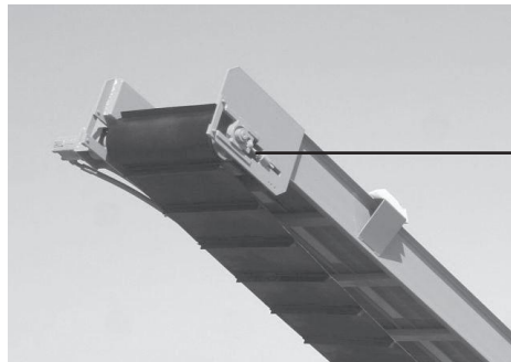
Figure 2.6 discharge conveyor belt adjusting bolts
