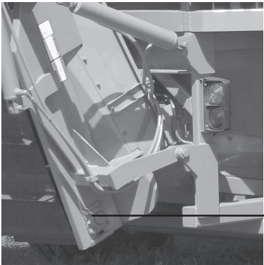
Figure 3.9 discharge conveyor bearings lubrication points (2 of 4)
