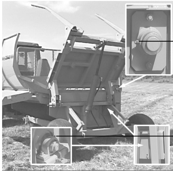
figure 4.4 slugbar adjustment bearing and rotor bearing lubrication points
