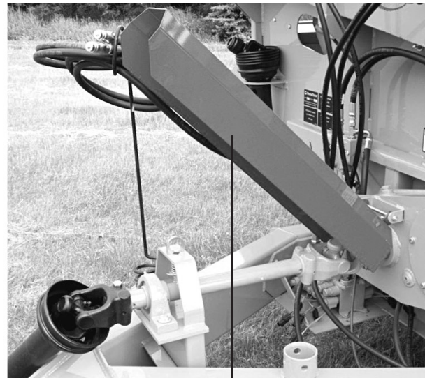
P.T.O. shield maintenance (raised) position
