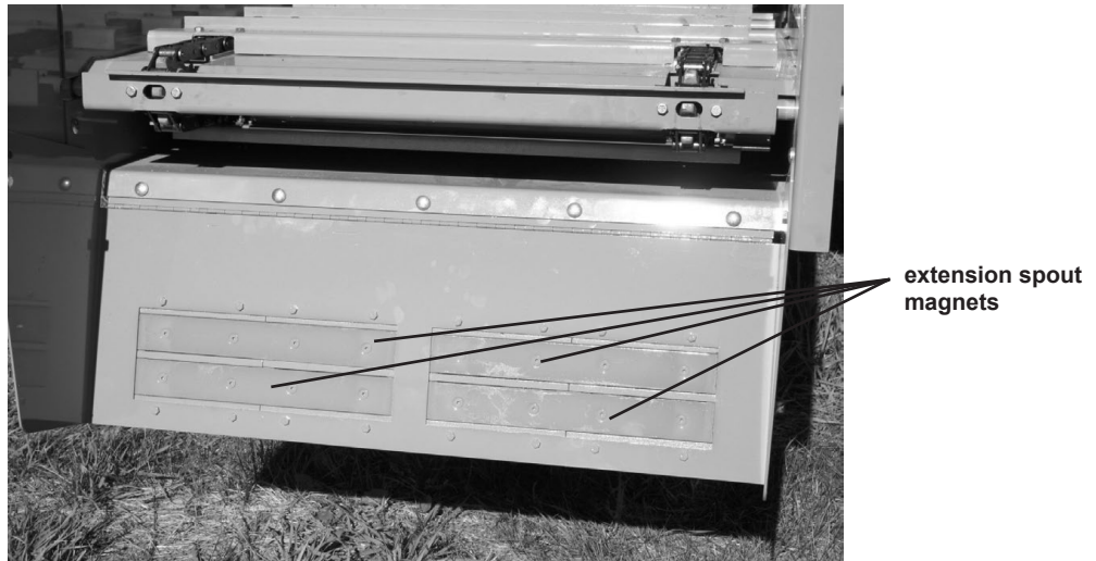
figure 6.2 Magnetic extension spout
