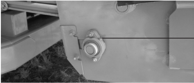
figure 4.8 Extention conveyor bearings lubrication point (1 of 4)
