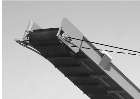
discharge conveyor bearing lube points
