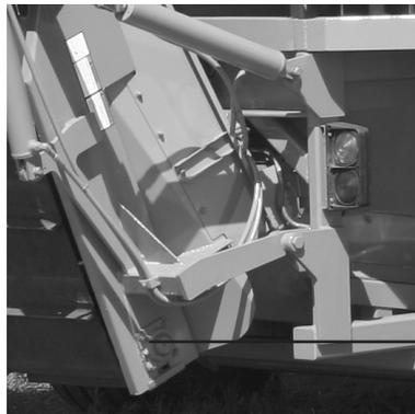
discharge conveyor bearing lube points
