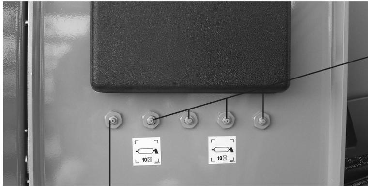
belly auger bearing lubrication
