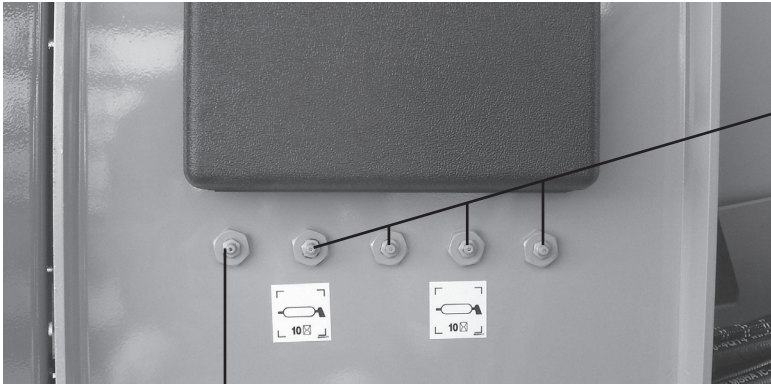
Figure 3.2 rotor bearing and belly auger bearing lubrication points
