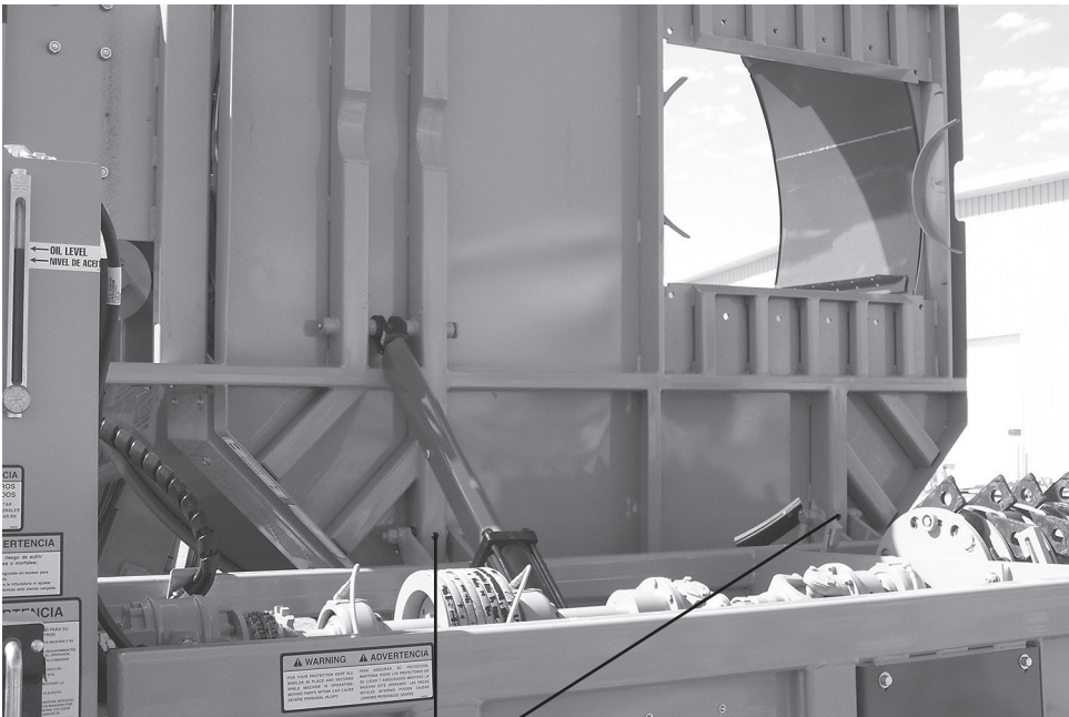
tub pivot lubrication points (Ref #4)
