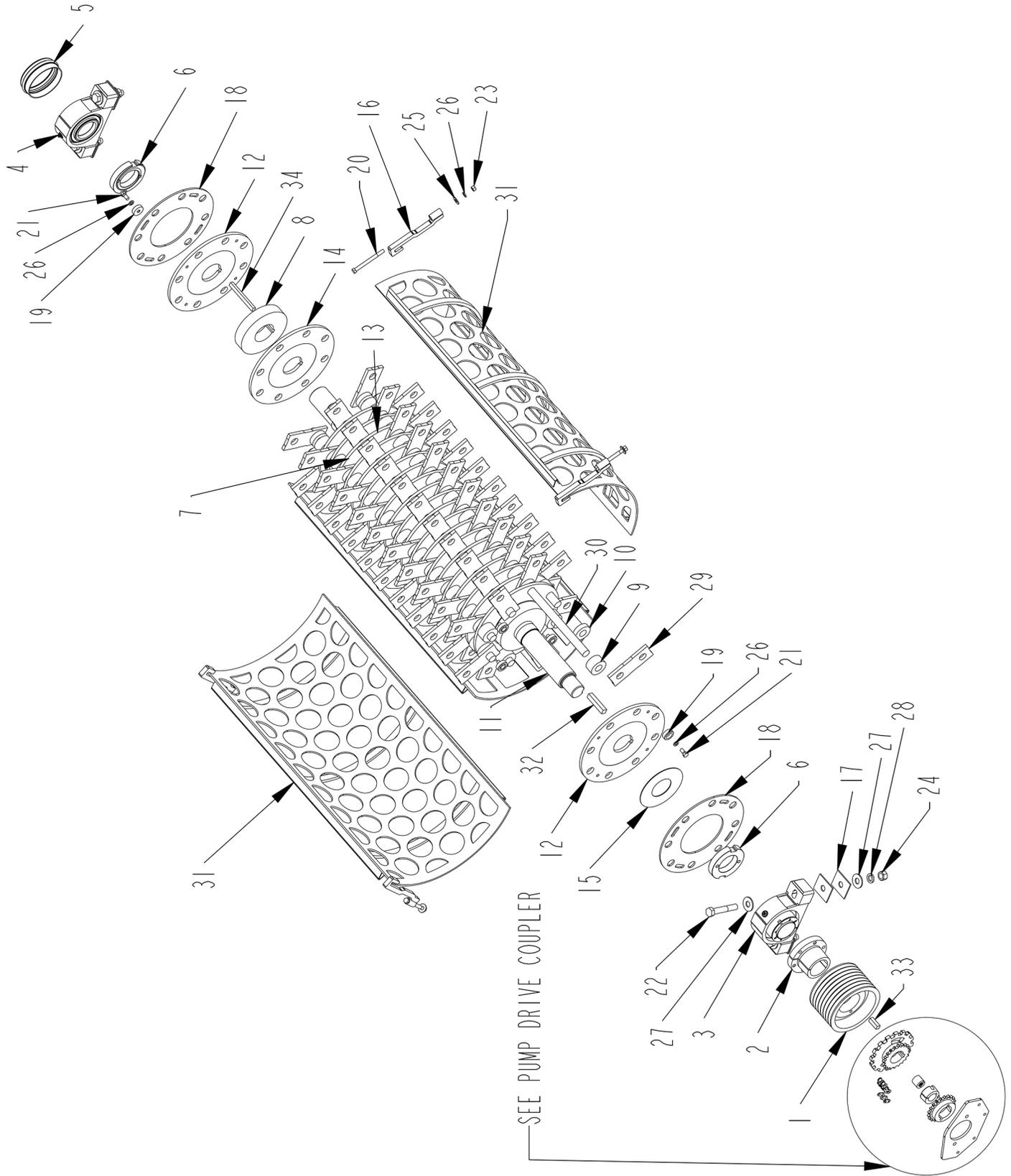
**ROTOR ASSEMBLY (S.N. 1111022030 UP TO 1117090030)**
