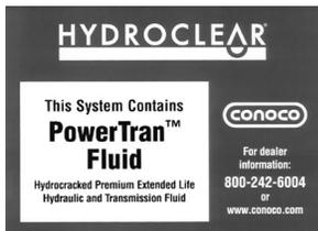
DuraTech Industries recommends using Cenex Qwicklift HTB if your machine has a Qwicklift decal on the hydraulic tank. Other acceptable fluids include Mobil 423, Farmland Super HTB, Conoco Hydroclear Power Tran Fluid, or other similar fluids. If the hydraulic tank does not have a decal, then all the above fluids are acceptable.
