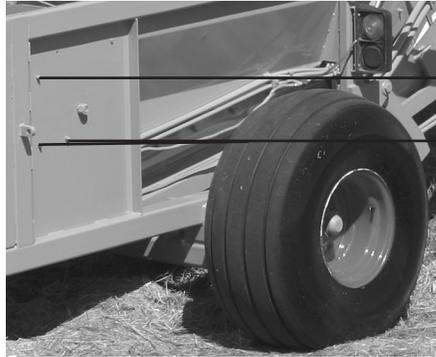
**front rotor bearing lubrication points 1 of 2 (Ref # 3)**
