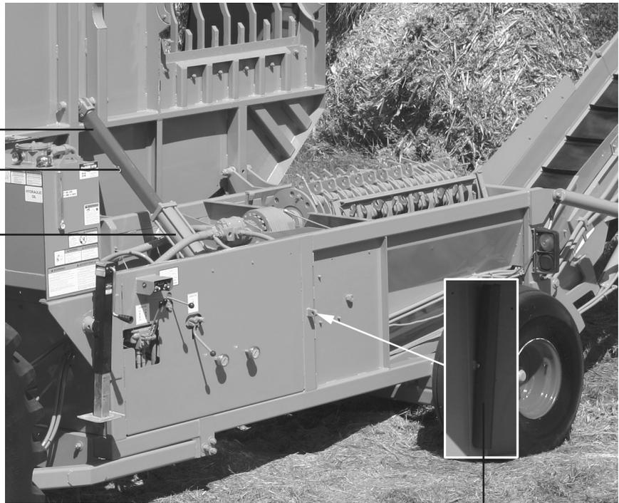
tub cylinder stop on storage bracket
