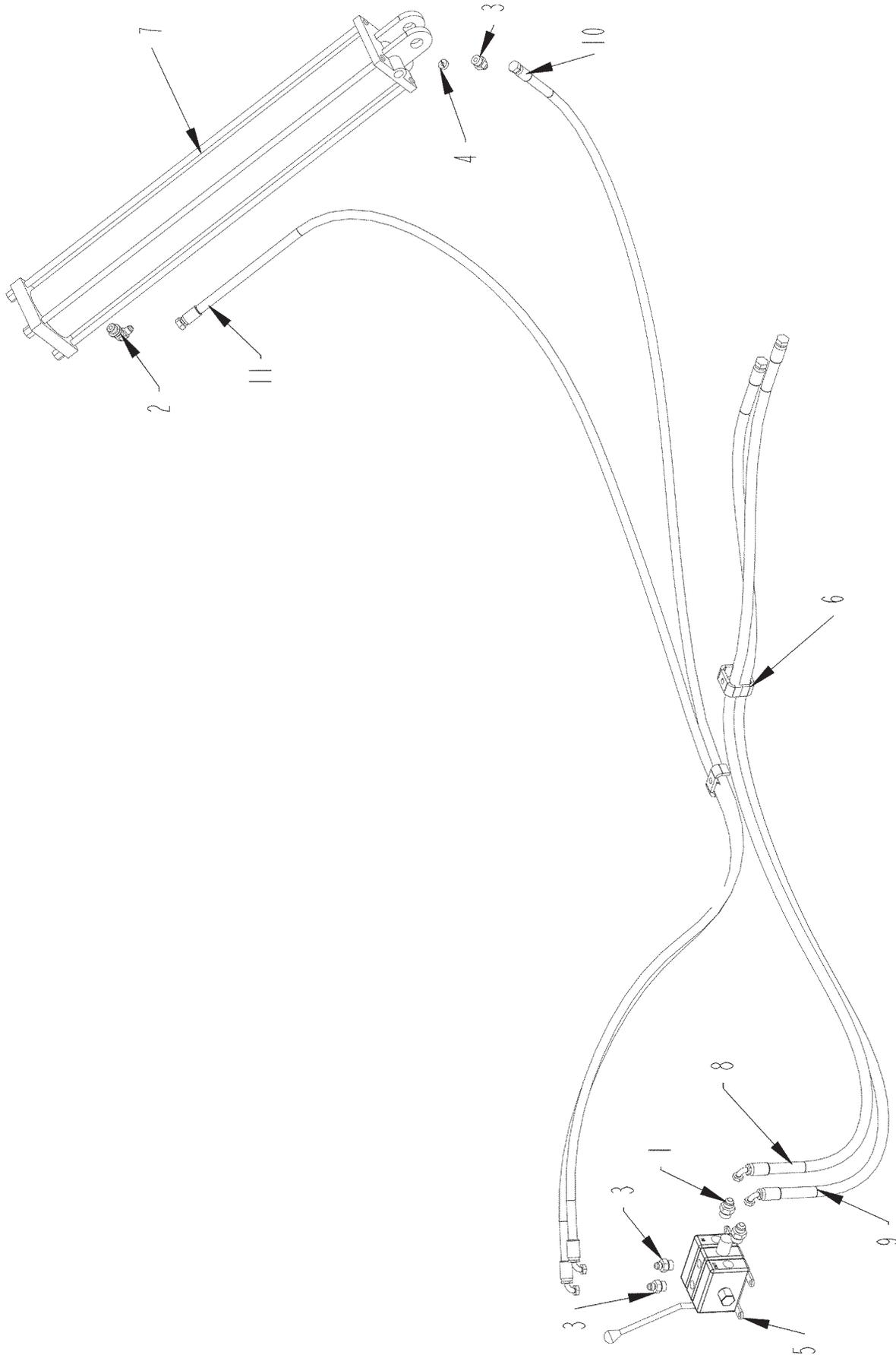
**TUB PLATFORM VALVE HYDRAULICS**
