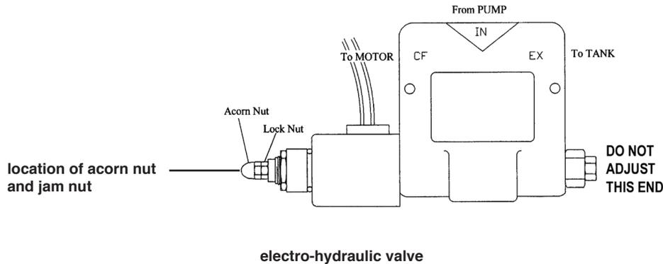
To calibrate the electro-hydraulic valve coil after following the three steps above, perform the following steps:
