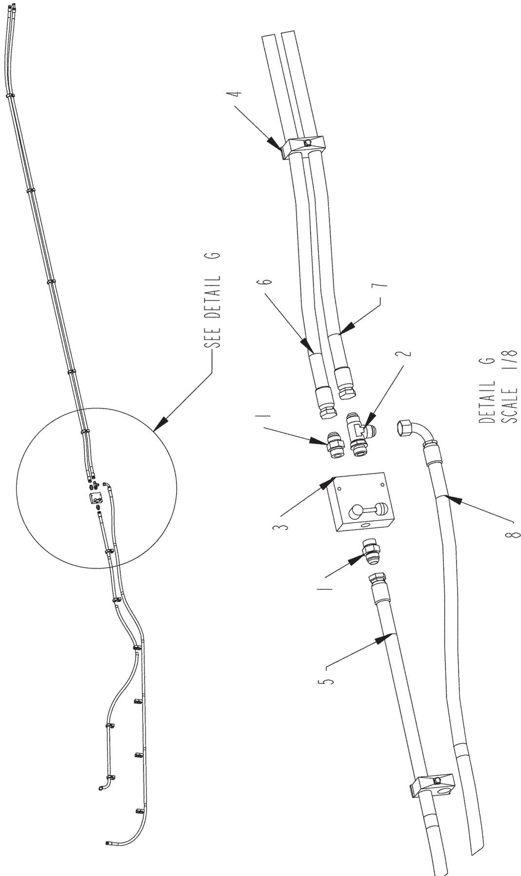
**CONVEYOR FLOW CONTROL VALVE HYDRAULICS (S.N. 1113040130 AND UP)**
