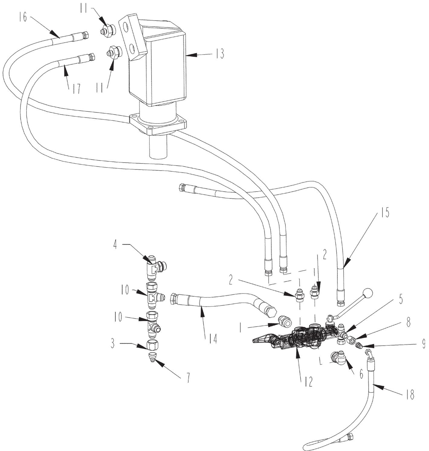
**TUB ROTATION VALVE AND TUB ORBIT MOTOR (S.N. 1110010130 AND UP)**
