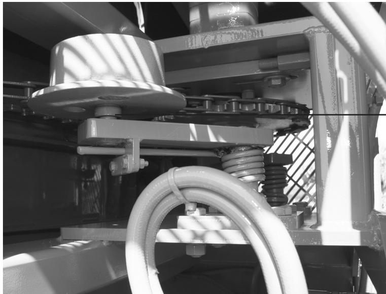
**tub chain idler pivot lubrication point (Ref #2)**
