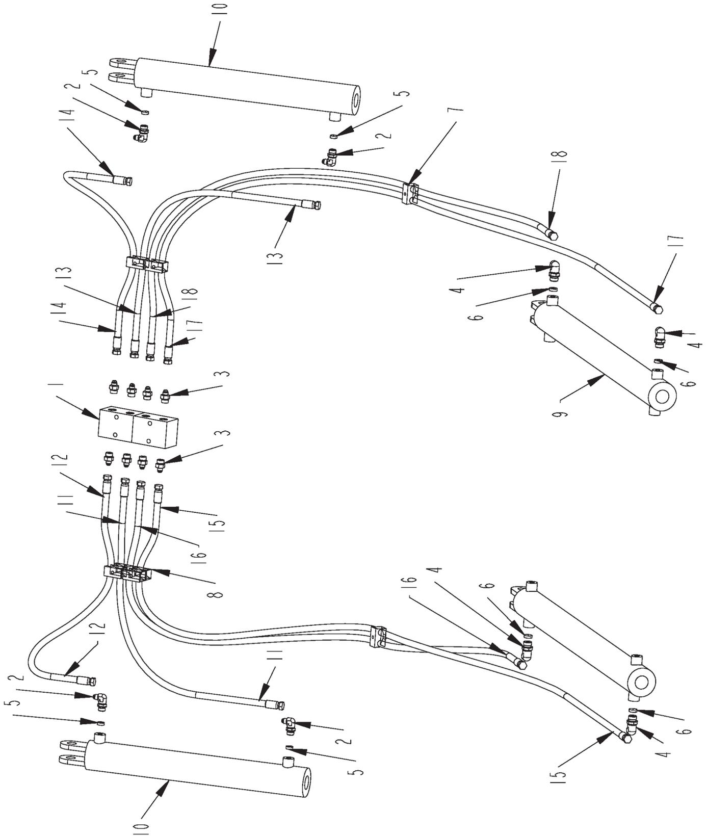
**CONVEYOR LIFT AND FOLD CYLINDER HYDRAULICS**
