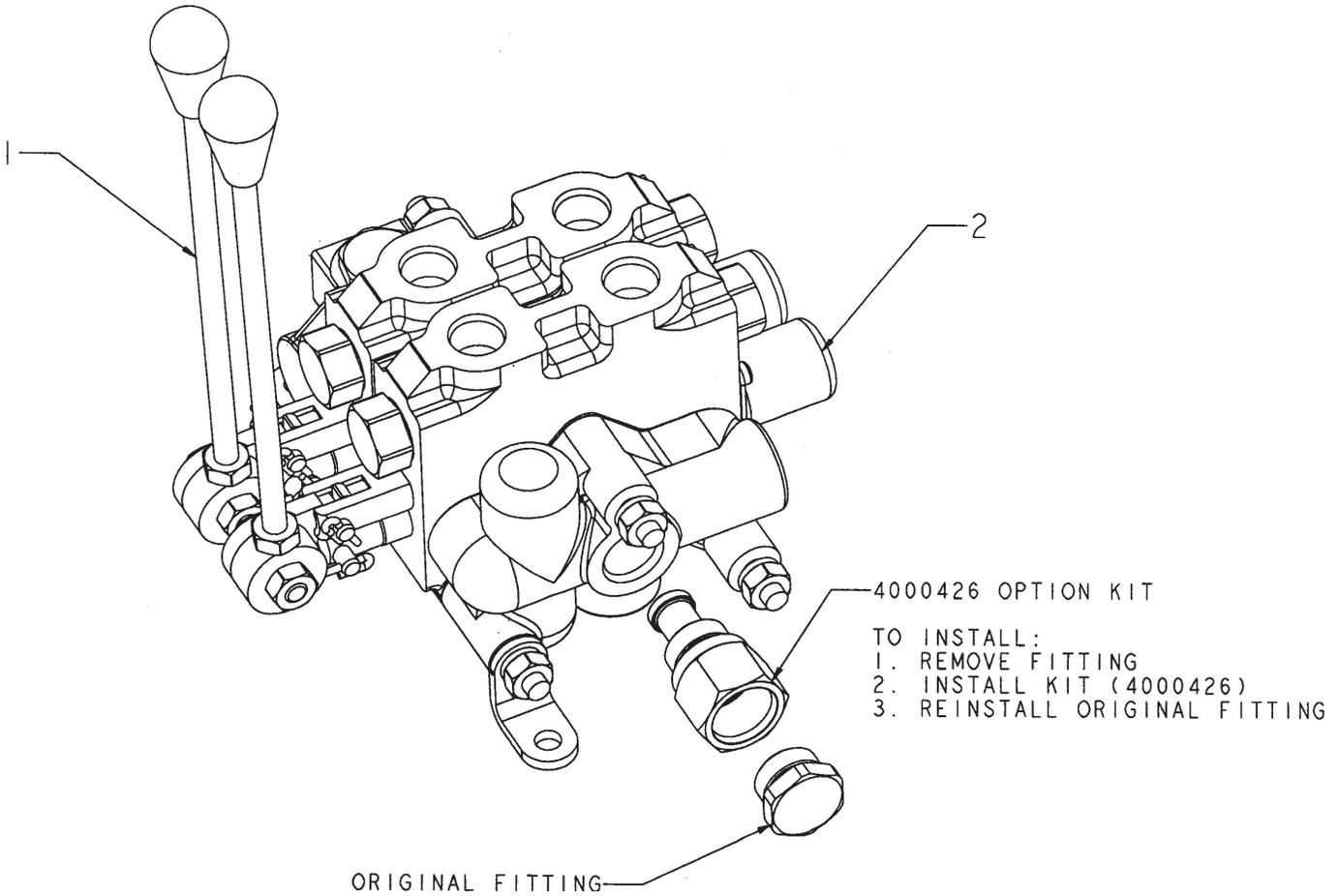
**MACHINE HYDRAULICS SCHEMATIC**
