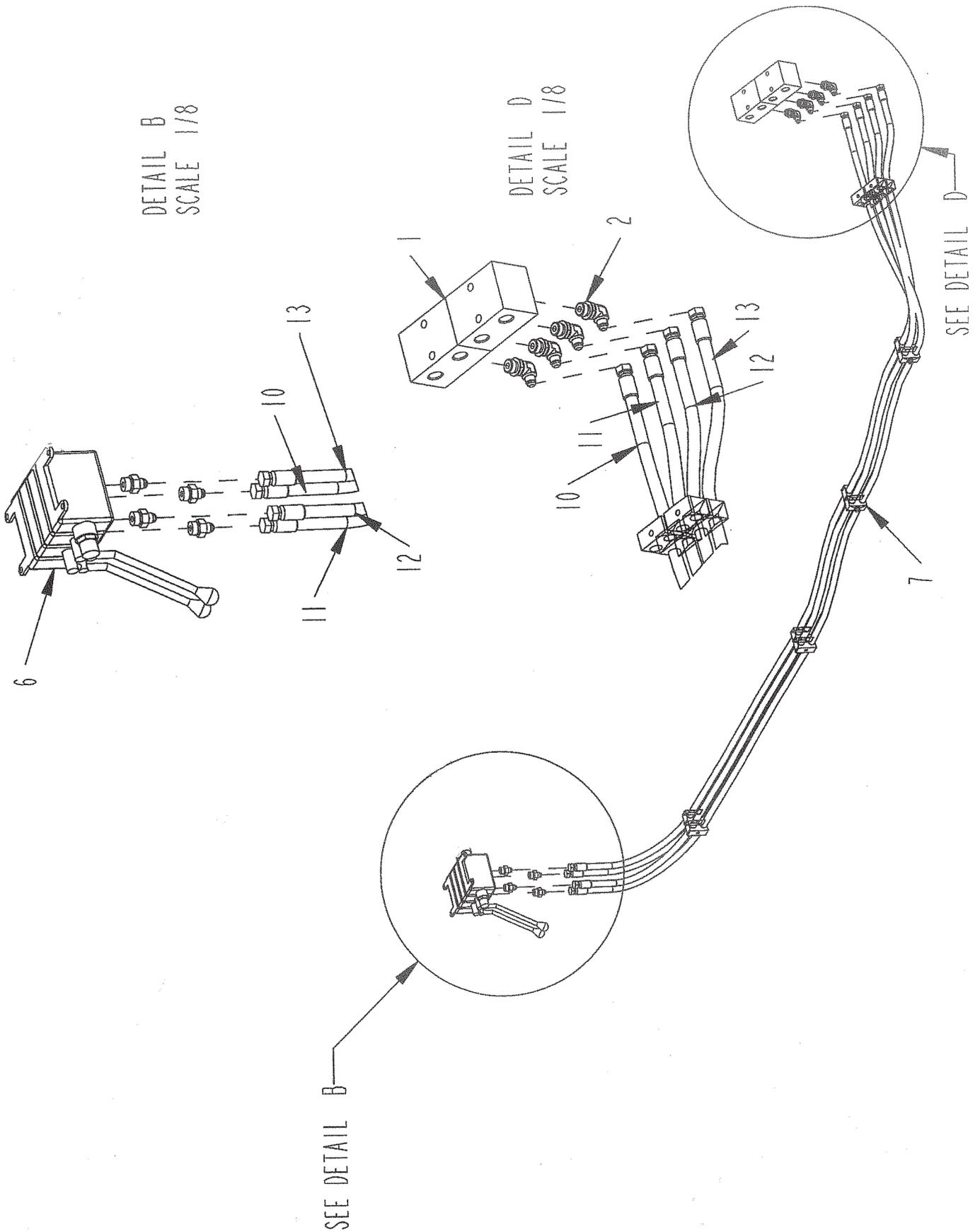
**CONVEYOR FOLD/UNFOLD & RAISE/LOWER VALVE HYDRAULICS
