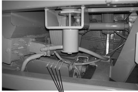
belly auger bearing lubrication points (Ref #5)
