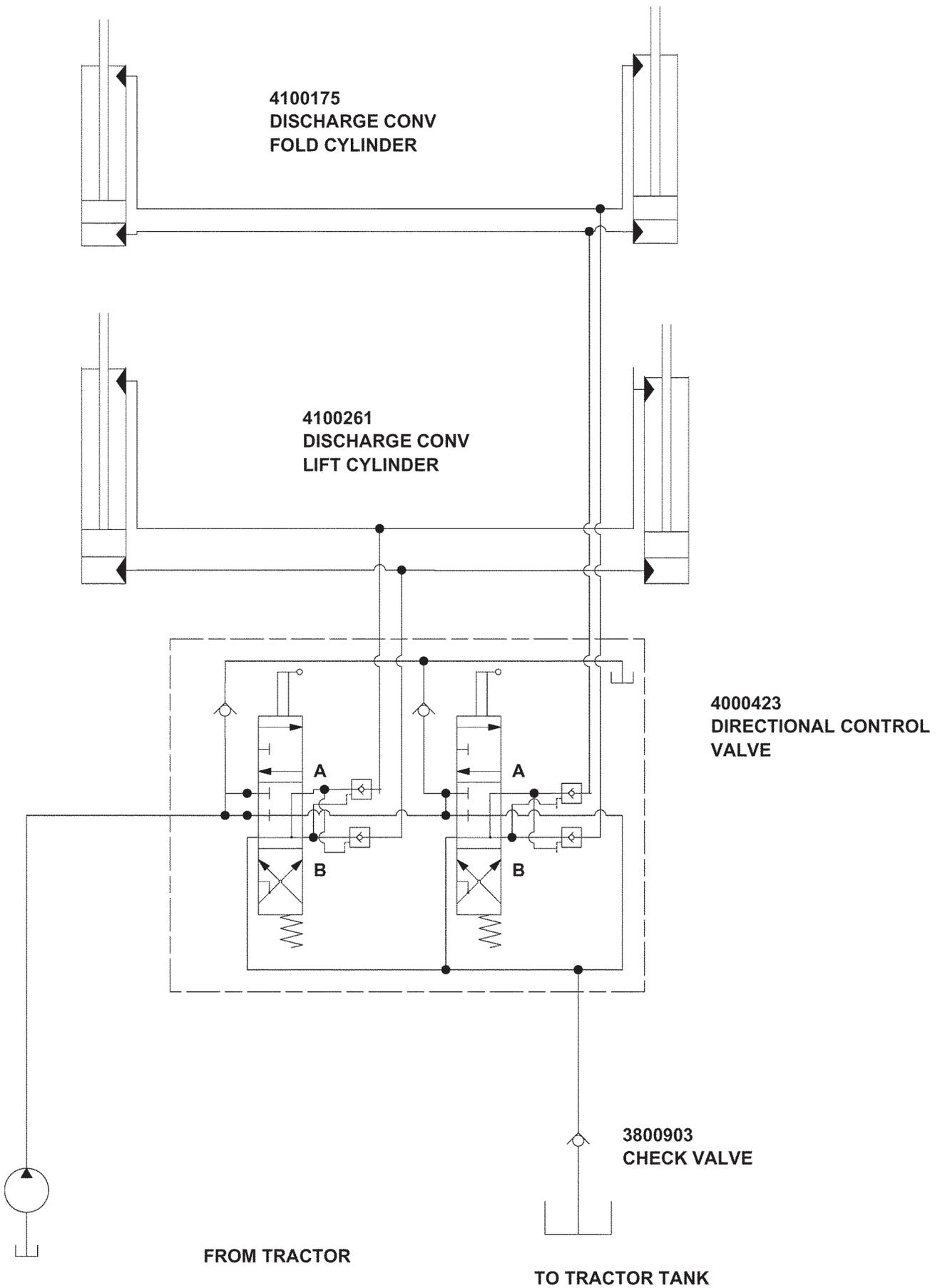
**TUB / CONVEYOR HYDRAULIC CIRCUIT**
