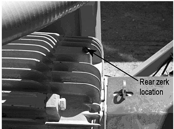
The P.T.O. shaft has (3) grease zerks that need to be lubricated every 40 hours. These locations are shown below.
