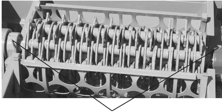
**rotor bearing lubrication points**
