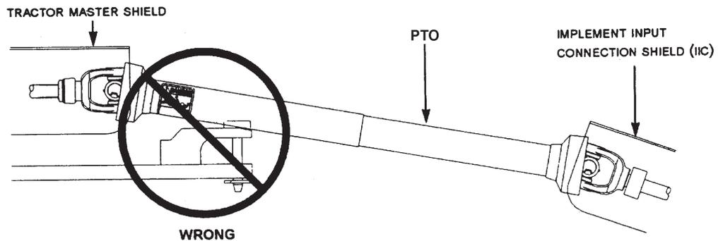
If this implement is attached to a tractor with an offset in the drawbar, be certain it is in the down position to prevent damage to the IID guarding and the IID telescoping members. See Figure 2.3.
