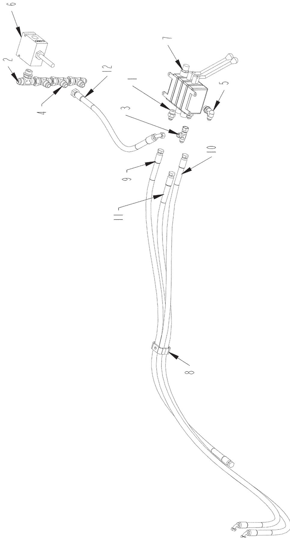
**CONVEYOR FOLD/UNFOLD & RAISE/LOWER VALVE HYDRAULICS**
