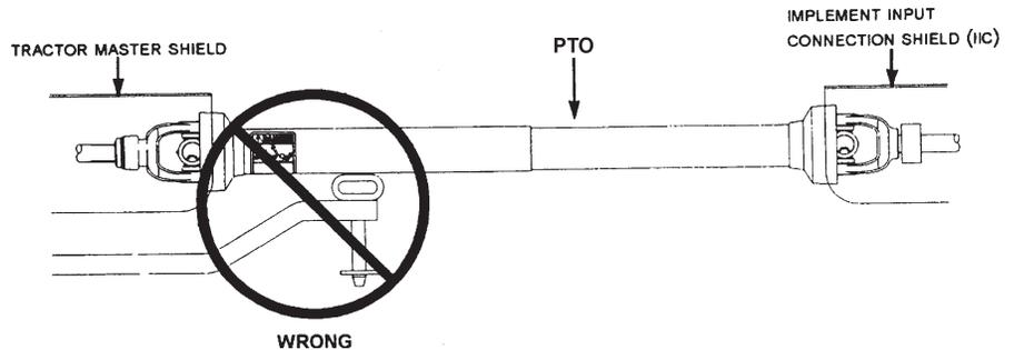
If this implement is attached to a tractor with 3-point arms, the arms must be fully raised and locked in position to prevent damage to the PTO guarding and the telescoping members. Adjust the tractor drawbar so the distance from the end of the PTO shaft on the tractor to the center of the drawbar hitch pin hole is 16" (41 cm.) for a 1-3/8" shaft, or 20" (51 cm.) for a 1-3/4" shaft, as shown in the illustration to the right.
