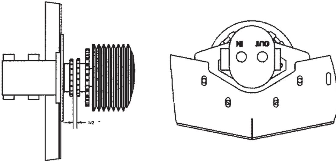
The chain coupler which transfers power from the rotor to the hydraulic pump will need to be removed if new belts are installed, a new hydraulic pump is installed, or if the rotor is removed. It is important to correctly install the coupler, if not the hydraulic pump shaft will be stressed and cause pump failure. To correctly install the coupler follow these step by step instructions.
