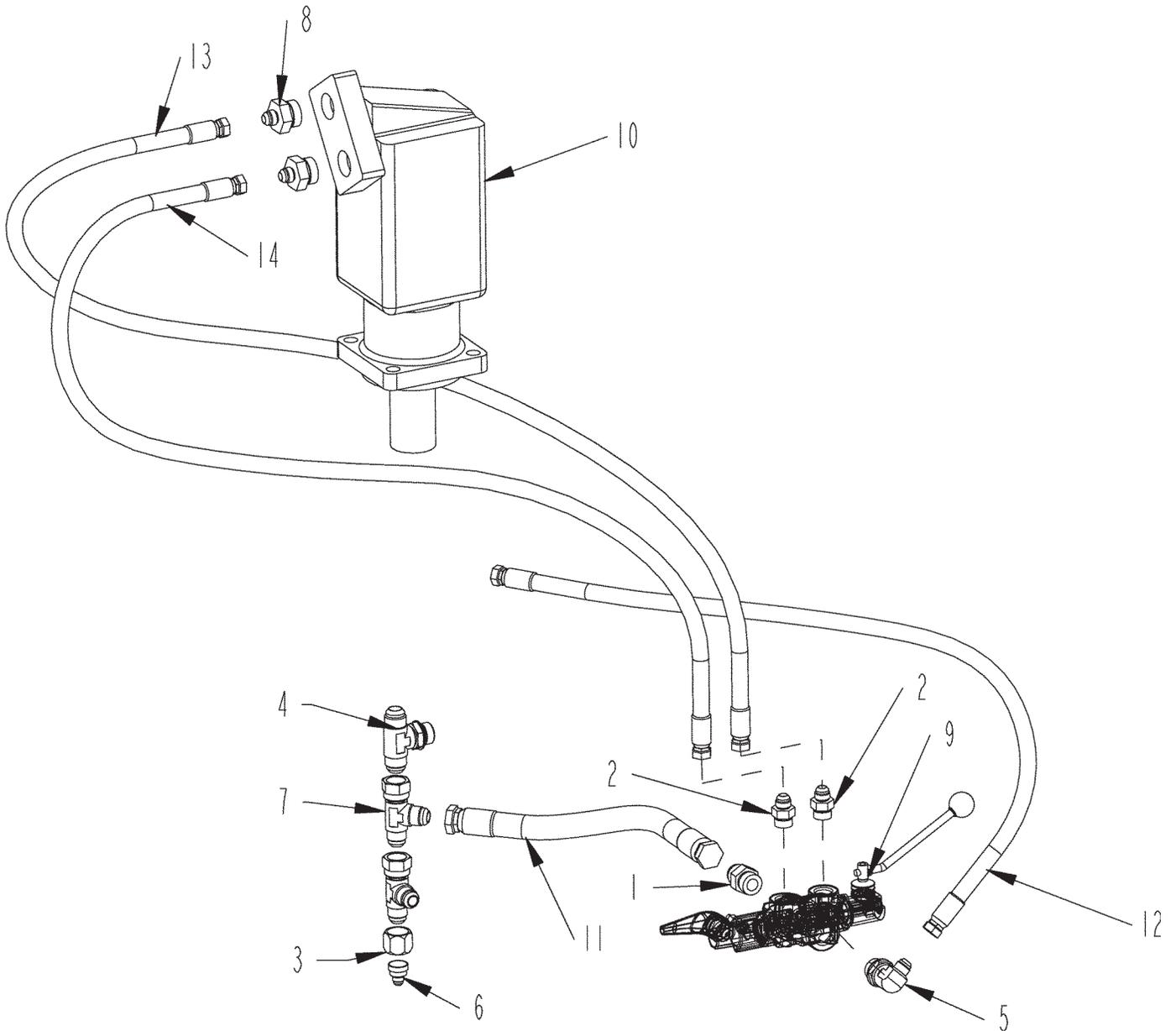
**TUB ROTATION VALVE AND TUB ORBIT MOTOR (S.N. UP TO 1110010030)**
