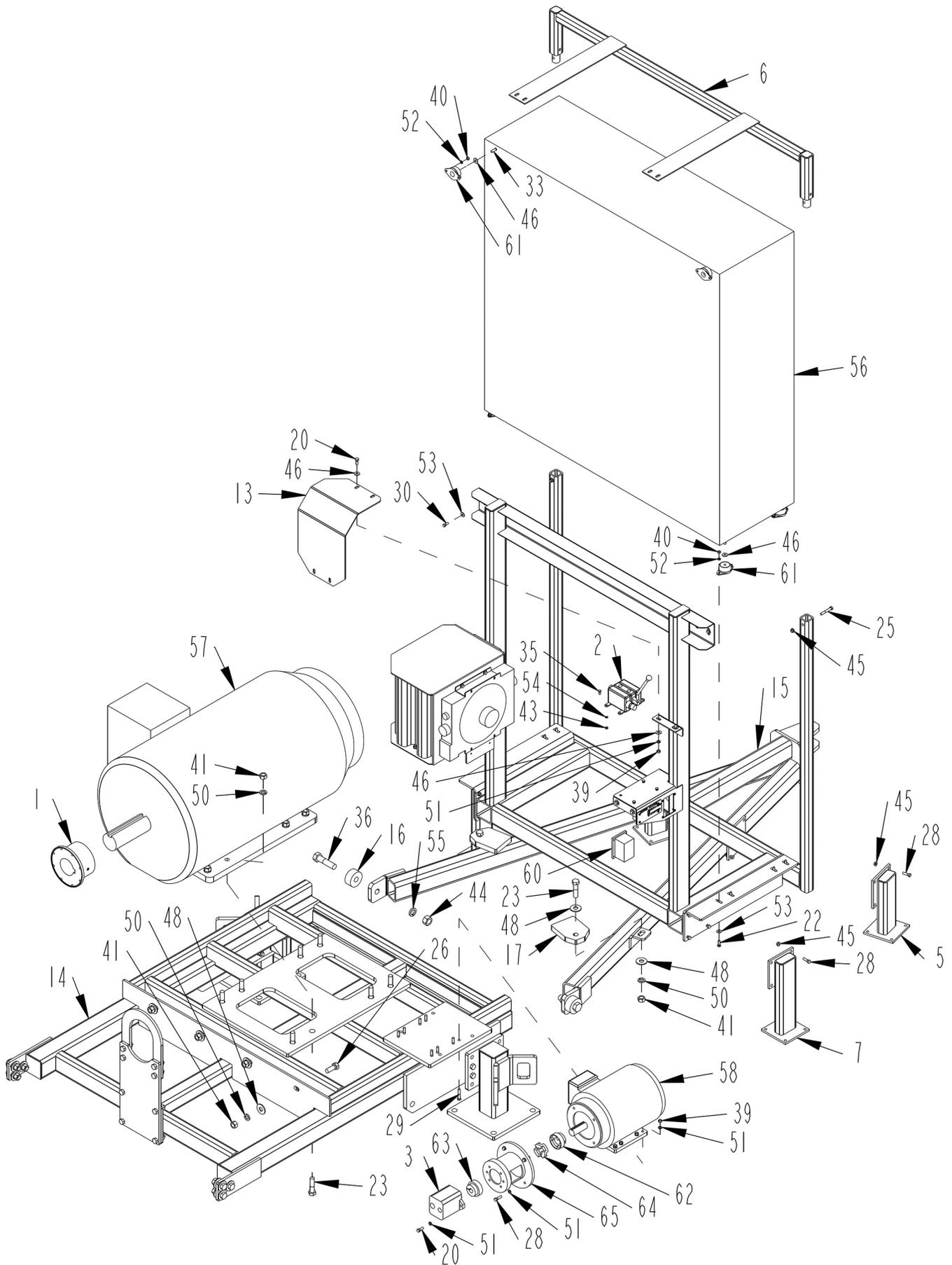
**ELECTRIC MOTOR ASSEMBLY #1 (S.N. 0651 & UP)**
