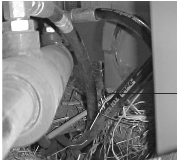
figure 5.2 rotor bearing vent and sight glass
