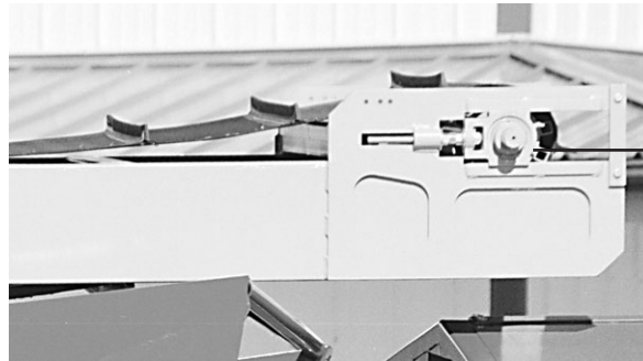
figure 5.6 discharge conveyor roller lubrication point
