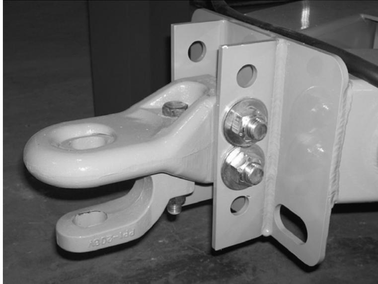
The hitch pin should be of proper diameter to prevent movement and length to extend through all components of the hitch. The pin should be secured with a hairpin clip or suitable device to prevent the loss of the pin.
