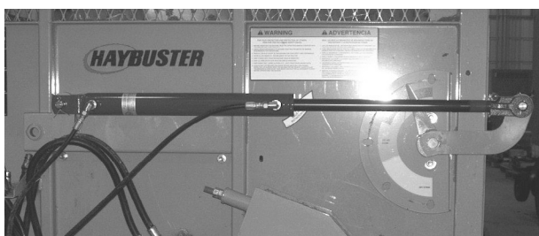
Hydraulic slug bar cylinder shown in the highest raised position
