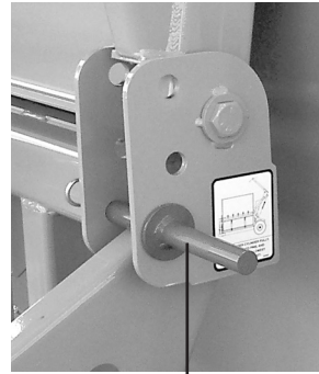
loader transport pin in storage position
