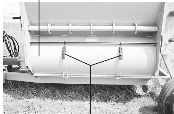
clean out door latches
