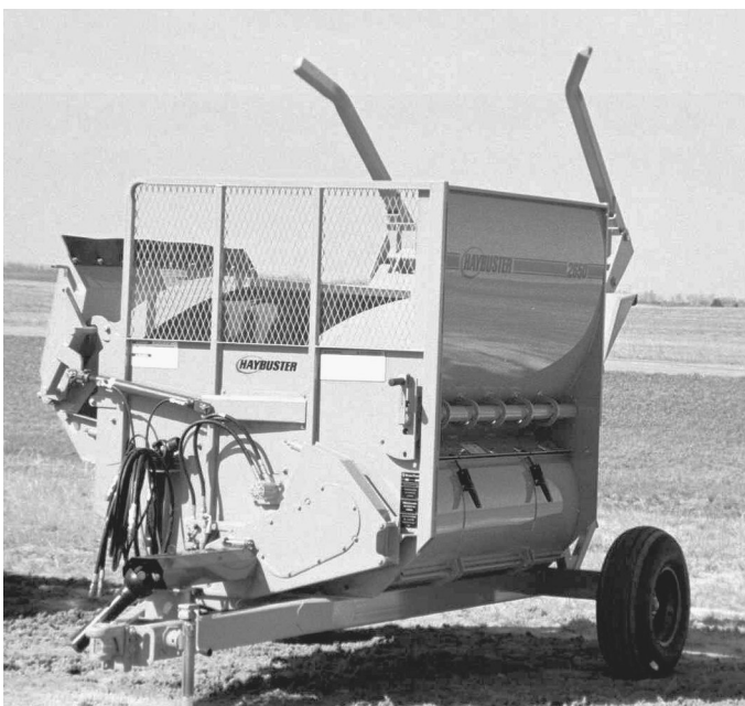
Rack and deflector in transport position
