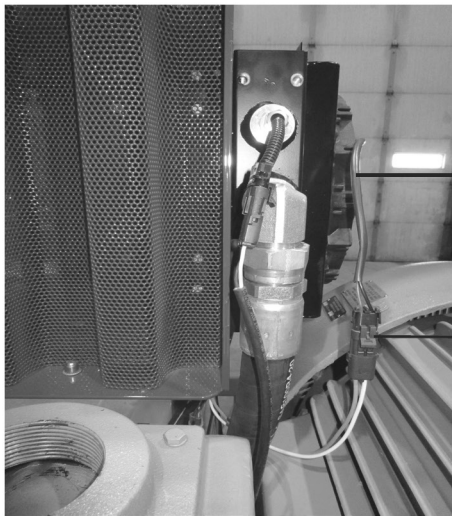
Figure 13 Disconnect fan from fan controller
