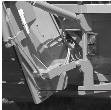
Figure 3.9 discharge conveyor bearings lubrication points (2 of 4)
