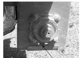
idler roller tension adjusting bolt
