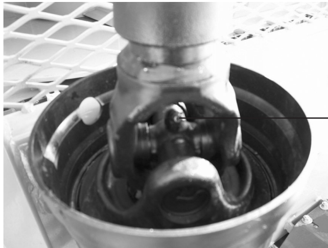
P.T.O. universal joint lubrication zerk
