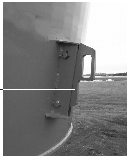
figure 3.4 Vertical knife adjustments, shown with knife in the fully engaged position
