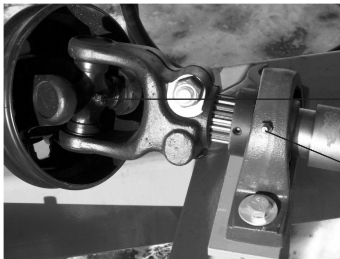
P.T.O. universal joint lubrication zerk
