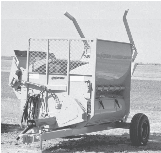
Rack and deflector in transport position
