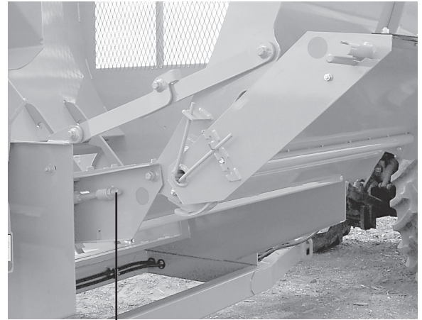
left conveyor chain adjustment bolt
