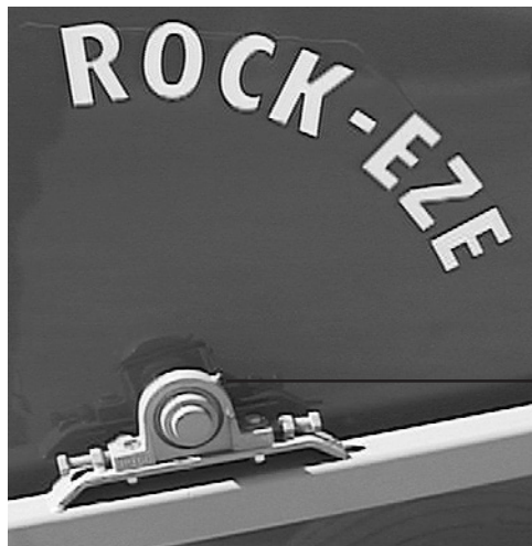
Rock wheel bearing lubrication zerk 1 of 2
