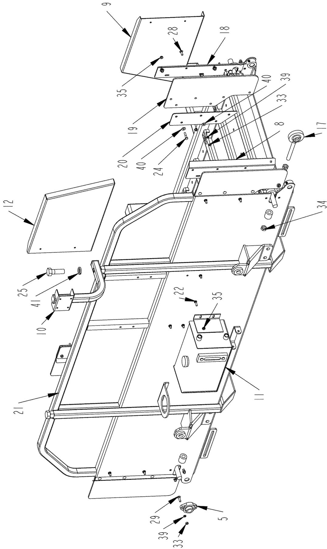
RIGHT HAND MAIN CONVEYOR ASSEMBLY-4704973 (SUB-ASSEMBLY 2)
