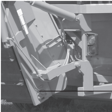
Figure 3.9 discharge conveyor bearings lubrication points (2 of 4)
