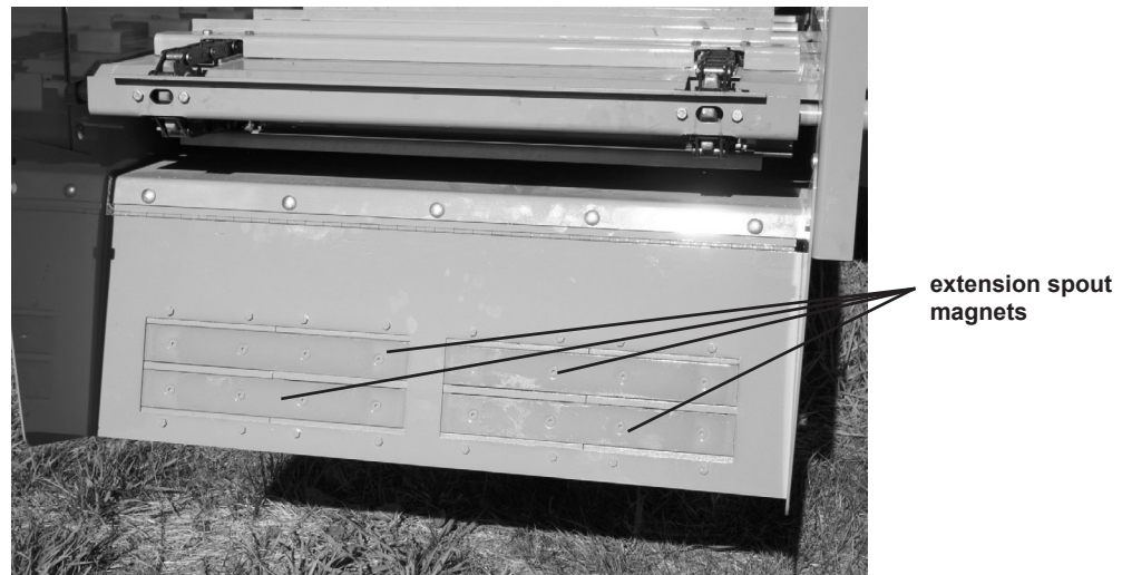
figure 6.2 Magnetic extension spout
