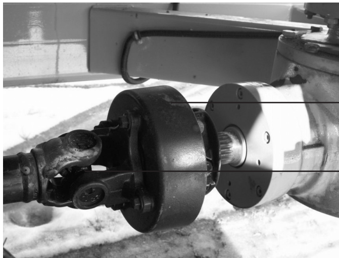
figure 4.6 P.T.O. Universal joint (8 of 8), and automatic clutch
