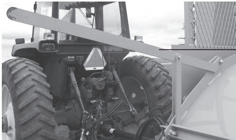
Rack tool in position for unfolding rack from transport position
