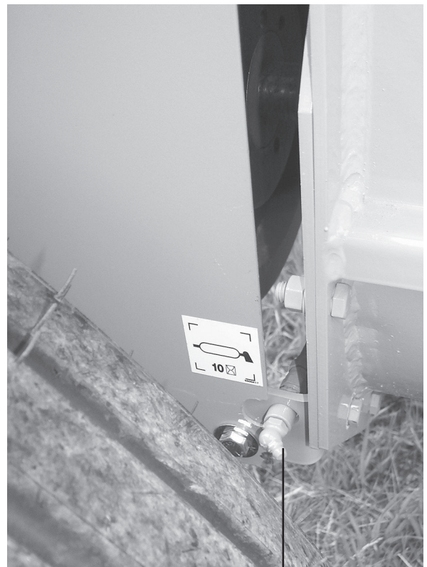
Auger bearing lubrication point
