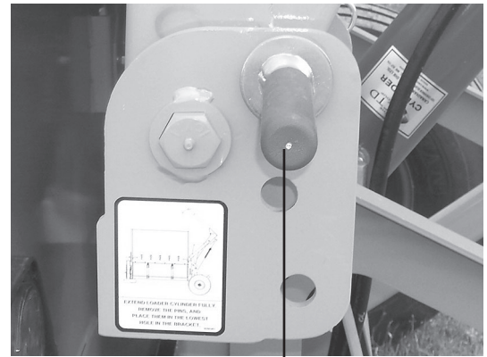
loader transport pin in transport position
