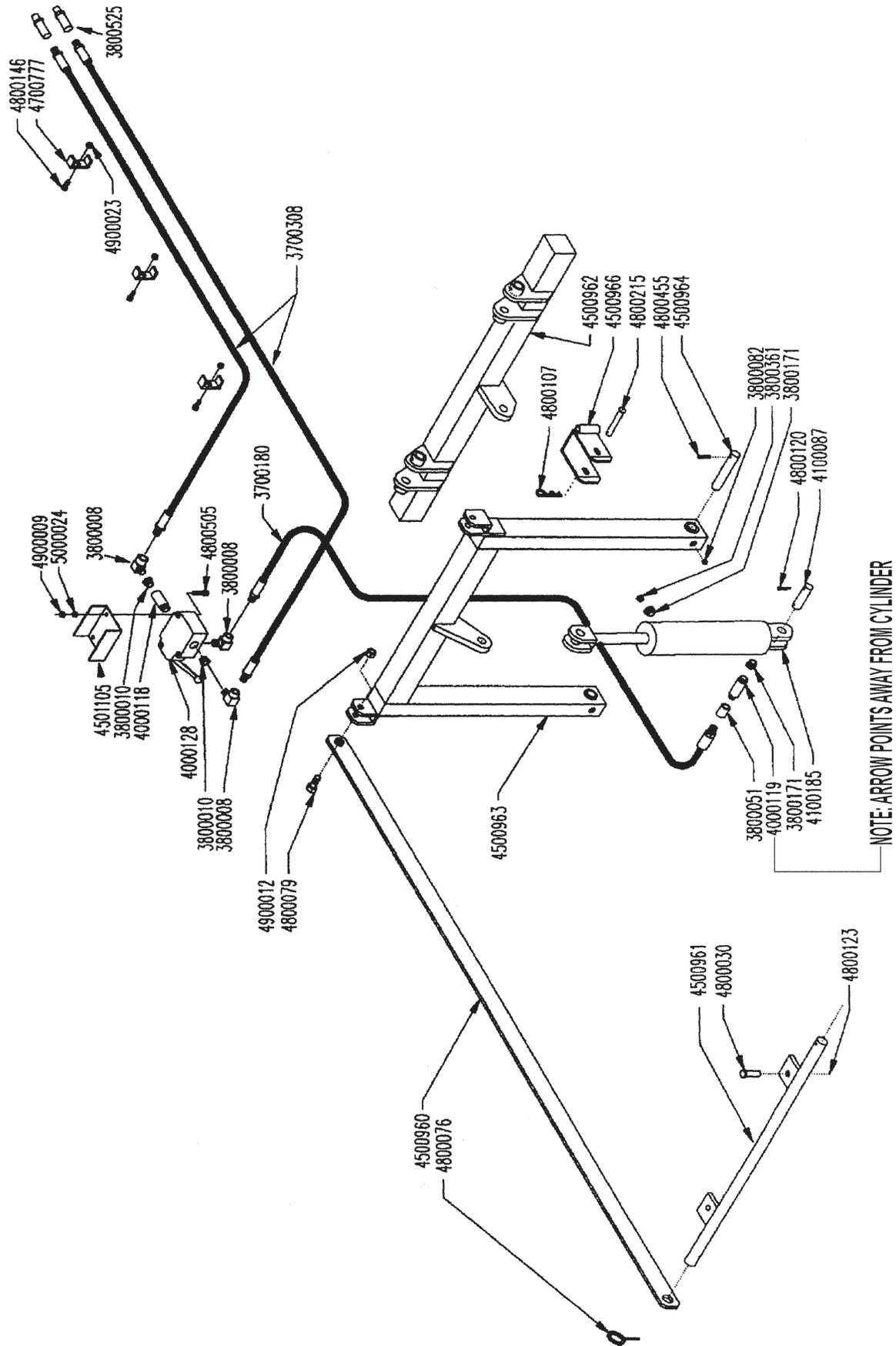
**HYDRAULIC CONVEYOR LIFT ASSEMBLY S.N. GI3757 TO GI3806**
