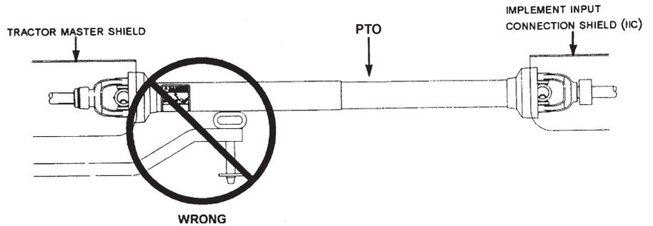
If this implement is attached to a tractor with 3-point arms, the arms must be fully raised and locked in position to prevent damage to the PTO guarding and the telescoping members. Adjust the tractor drawbar so the distance from the end of the PTO shaft on the tractor to the center of the drawbar hitch pin hole is 16" (41 cm.) for a 1000 RPM shaft as shown at right.
