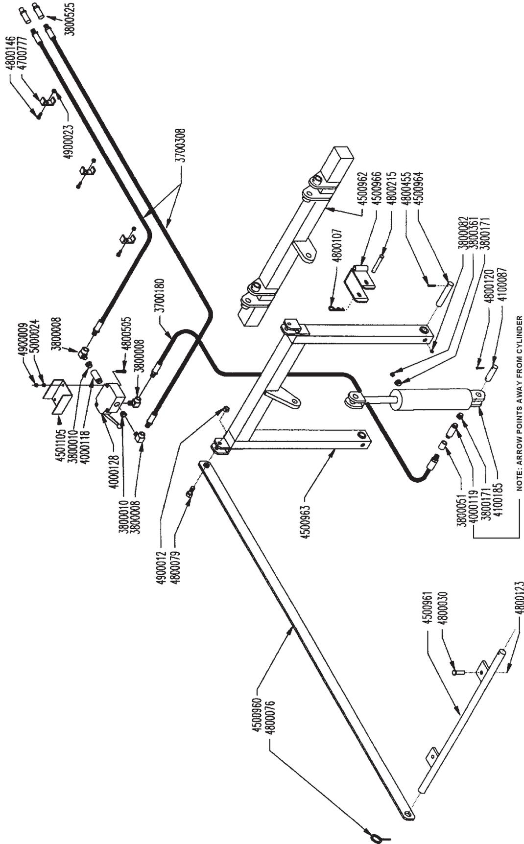
**HYDRAULIC CONVEYOR LIFT ASSEMBLY S.N. GI3807 AND UP**
