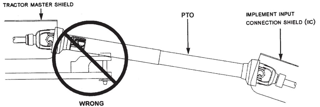
If this implement is attached to a tractor with an offset in the drawbar, be certain it is in the down position to prevent damage to the IID guarding and the IID telescoping members. See Figure 3.3.
