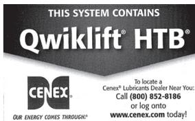
DuraTech Industries recommends using Cenex Qwiklift HTB if your machine has a Qwiklift decal on the hydraulic tank. Other acceptable fluids include Mobil 423, Farmland Super HTB, Conoco Hydroclear Power Tran Fluid, or other similar fluids. If the hydraulic tank does not have this decal, then all of the above fluids are acceptable.
