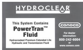
Approximately 6 gallons of hydraulic oil. DuraTech Industries recommends using Cenex Qwicklift HTB if your machine has a Qwicklift decal on the hydraulic tank. Other acceptable fluids include Mobil 423, Farmland Super HTB, Conoco Hydroclear Power Tran Fluid, or other similar fluids. If the hydraulic tank does not have this decal, then all of the above fluids are acceptable
