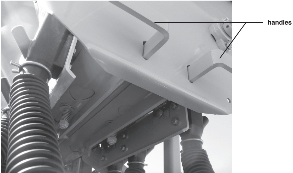
drill cleanout slides
