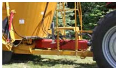
**CV PTO OR OPTIONAL 2-SPEED GEAR BOX:** The CMF-430 comes equipped with either a Heavy-Duty Constant Velocity 540 rpm PTO or an optional 2-Speed Gear Box. The 2-Speed Gear Box is used for loaded start-ups and heavy rations.
