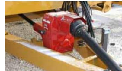
**CV PTO OR OPTIONAL 2-SPEED GEAR BOX:** The CMF-830 comes equipped with either a heavy-duty constant velocity 1000 rpm PTO or an optional 2-speed gearbox. The 2-speed gearbox is used for loaded startups and heavy rations.
