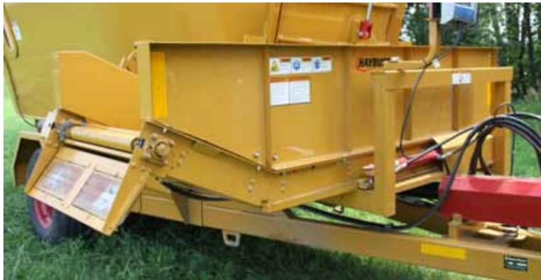
**DOGLEG CONVEYOR:** The dogleg style conveyor hydraulically slides out 16" for easy access to feed bunks.
