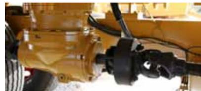
**CLUTCH:** Free motion clutches on the driveline protect the heavy-duty gear boxes. Gear boxes come with a 2-year warranty. The optional 2-speed gear box is used for loaded start-ups and heavy rations.
