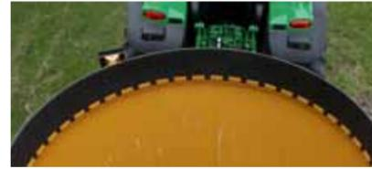
**RUBBER EXTENSION:** The tapered boiler ring is standard equipment on the CMF-430. It prevents product from boiling over the sides during the cutting and mixing processes.
