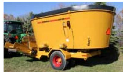
**HEAVY-DUTY FRAME:** The CMF-830 is built with a heavy-duty 6" x 9" x ¼" steel tube frame for strength and durability.
