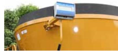
**DIGI-STAR:** The CMF-430 is equipped with a Digi-Star 4 pt. scale and monitor. Various monitor options are available. The Digi-Star system is powered by a standard onboard 12-volt battery. Digi-Star feed rationing programs are also available.
