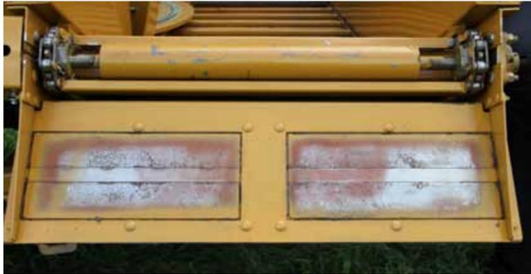
**MAGNETS ON CHUTES:** Magnets on the discharge chutes removes metal, such as bale wire from feed, providing the highest quality feed available. Standard on the dogleg conveyor.
