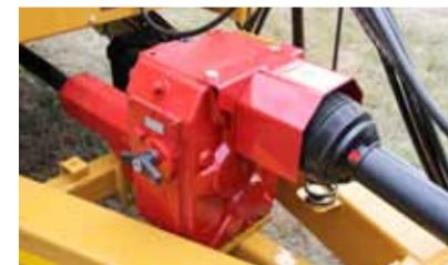
**CV PTO WITH 2-SPEED GEAR BOX:** The CMF-980 comes equipped with a heavy-duty 1 3/4" constant velocity 1000 rpm PTO with a 2-speed gearbox. The 2-speed gearbox is needed for loaded startups and heavy rations.
