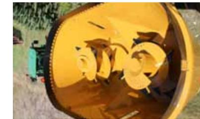
**AUGERS:** Heavy-duty 88" screw augers with 18-1/4" self-sharpening serrated knives, driven by 2 HD USA gearboxes.
