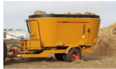
**MIXING CAPACITY:** The CMF-980 has a 980 cu. ft. mixing capacity with a tare weight of 30,900 lbs.
