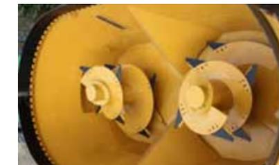
**AUGERS:** Heavy-duty 88" screw augers with self-sharpening serrated knives, driven by 2 HD USA gearboxes.
