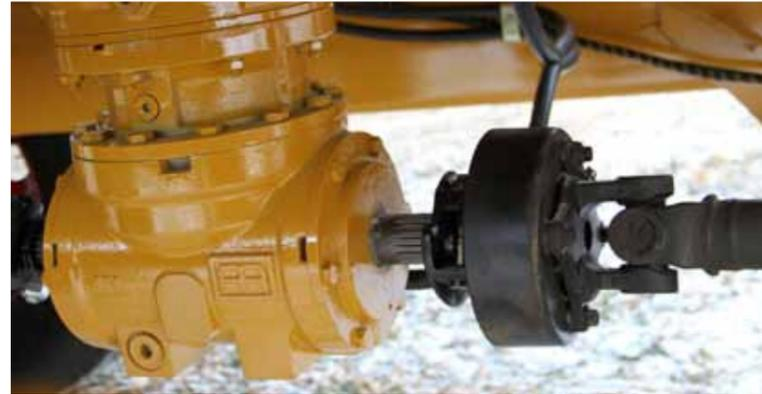
**FREE MOTION CLUTCHES ON DRIVELINE:** Free motion clutches on driveline protect the heavy duty gearboxes. Gearboxes come with a two-year warranty. The optional two-speed gearbox is used for loaded startups and heavy rations.
