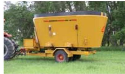
**MIXING CAPACITY:** The CMF-710 has a 710 cu. ft. mixing capacity with a tare weight of 18,340 lbs.
