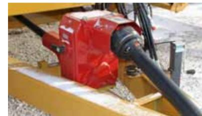
**CV PTO OR OPTIONAL 2-SPEED GEAR BOX:** The CMF-710 comes equipped with either a heavy-duty constant velocity 1000 rpm PTO or an optional 2-speed gearbox. The 2-speed gearbox is used for loaded startups and heavy rations.
