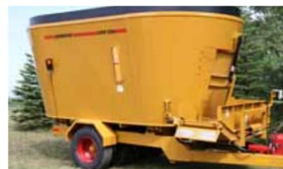
**HEAVY-DUTY FRAME:** The CMF-1150 is built with a heavy-duty 6" x 10" x 3/8" steel tube frame for strength and durability.
