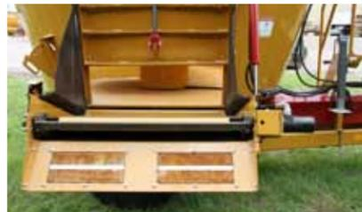
**MAGNETS:** Magnets on the discharge chutes remove metal, such as bale wire, from feed providing the highest quality feed available.
