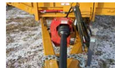
**CV PTO WITH 2-SPEED GEAR BOX:** The CMF-1150 comes equipped with a heavy-duty 1 3/4" constant velocity 1000 rpm PTO with a 2-speed gearbox. The 2-speed gearbox is needed for loaded startups and heavy rations.
