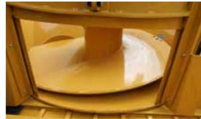
**UNLOADING DOOR:** Large 24" x 42" unloading door for fast, even unloading and clean-out.
