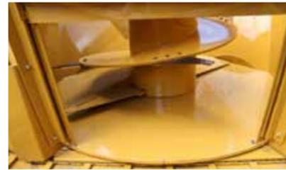
**UNLOADING DOOR:** Large 30" x 42" unloading door for fast, even unloading and clean-out.
