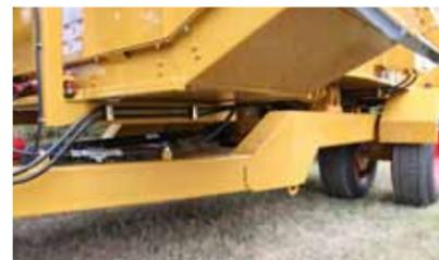
**HEAVY-DUTY FRAME:** The CMF-980 is built with a heavy-duty 6" x 10" x 3/8" steel tube frame for strength and durability.
