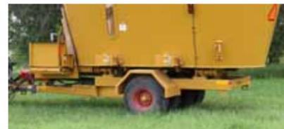
**HEAVY-DUTY FRAME:** The CMF-710 is built with a heavy-duty 6" x 9" x ¼" steel tube frame for strength and longevity.
