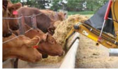
**CONVEYOR:** The unloading door is 42" high and can be on the left or right side of the machine. Conveyor options are a 3' or 5' extension which gives a feeding height range of between 36" and 58".
