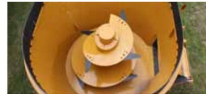
**AUGER WITH KNIVES:** 88" heavy-duty single auger with up to 7 self-sharpening serrated knives driven by an HD USA gearbox.
