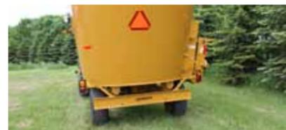
**RIGID AXLES:** Rigid heavy-duty axles on each side with 2 14L-16.1 12 ply tires.
