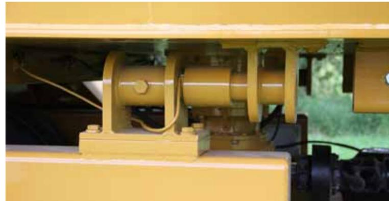
**4-POINT SCALE:** 4-point scale for accurate weighing, with reduced scale bounce during loading and feeding.
