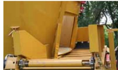
**UNLOADING DOOR:** Large 24" x 42" unloading door for fast, even unloading and cleaning.
