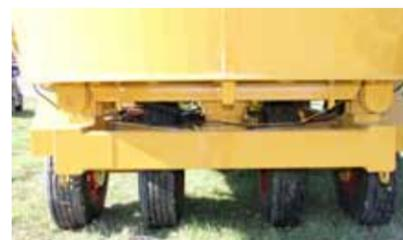
**OSCILLATING AXLES:** Oscillating Heavy Duty Axles with 4) 315/80 R 22.5 20-ply rated tires provide even weight distribution on uneven or frozen ground.
