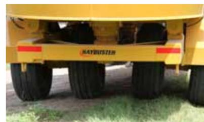
**OSCILLATING AXLES:** Oscillating Heavy Duty Axles with 4) 315/80 R 22.5 20-ply rated tires provide even weight distribution on uneven ground.
