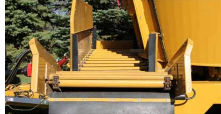
**VERSATILE 36 IN. WIDE CROSS AND UNLOADING CONVEYOR:**
