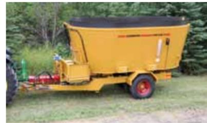
**MIXING CAPACITY:** The CMF-830 has an 830 cu. ft. mixing capacity with a tare weight of 21,500 lbs.
