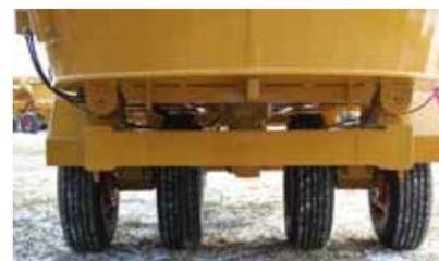
**OSCILLATING AXLES:** Oscillating Heavy Duty Axles with 4) 385/65 R 22 20-ply rated tires provide even weight distribution on uneven or frozen ground.
