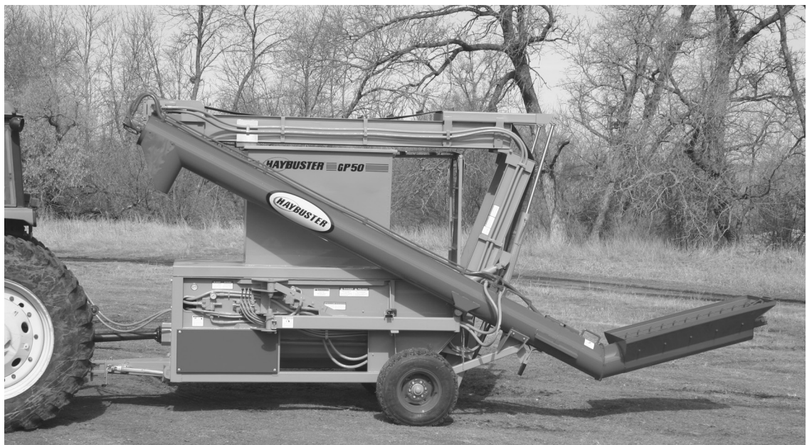
Figure 2.4 GP-50 Grain Processor shown in transport mode.
