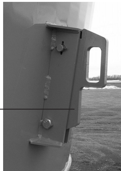
figure 3.4 Vertical knife adjustments, shown with knife in the fully engaged position
